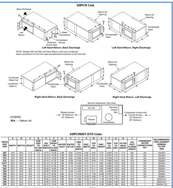
When waterside economizer is installed, increase width by 7 inches. When WSHP Open Controller is installed, increase depth by 2.6 inches. When waterside economizer is installed, increase depth by 7 inches. 50PCH015 units built with ECM motor option. +
