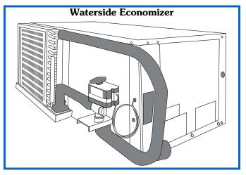
Water flow through the waterside economizer is controlled by a factory installed and wired 3-way motorized valve. When the waterside economizer is active (based on the Aquastat set point), flow is through the waterside economizer coil and then through the coaxial coil. When mechanical cooling is active (when the water loop temperature is outside the Aquastat set point), water flow is through the coaxial coil only.
